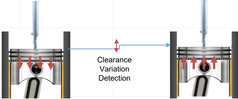
Piston Cylinder Expansion
